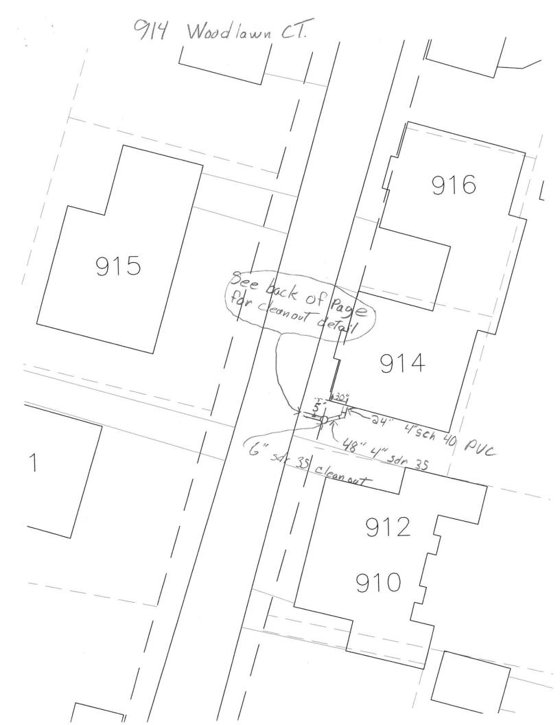
C'Lleonout oTgrade 6x4 Tee (4" sdr 35 To house See other Side 450 450 Existing 6" sdn 35 To city sewer -
